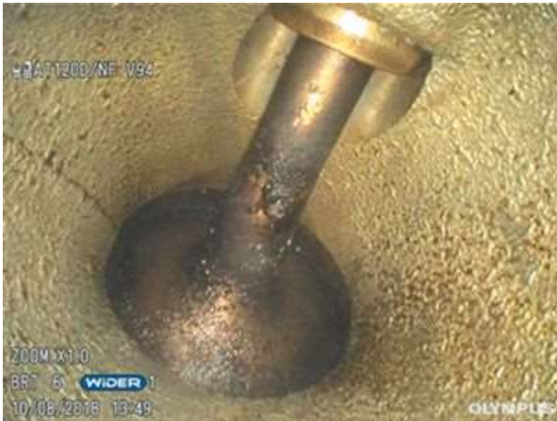
Figure 2: Example of carbon build-up on the engine valve as viewed through the IPLEX GX with 4 mm 120° direct-view near-focus tip adaptor.
