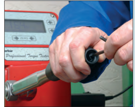
'P' Type wrenches have no scale. They must be set against a torque testing device such as Norbar's Professional Torque Tester (see page 68).
