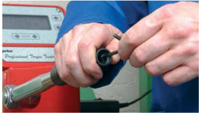
Setting a 'P' Type Torque Wrench
