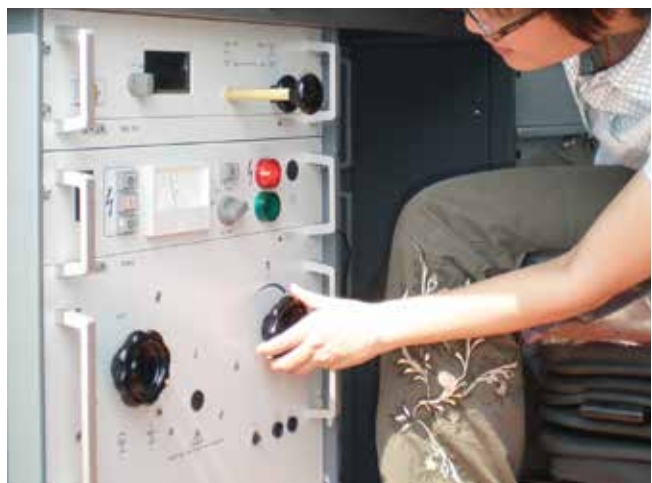
➤ setting of voltage and selection of voltage range at the surge generator SSG
