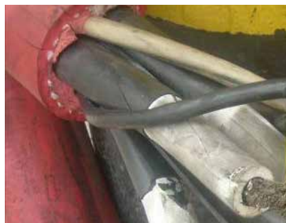
➤ 3-core EPR, incl. dataline, radial type
