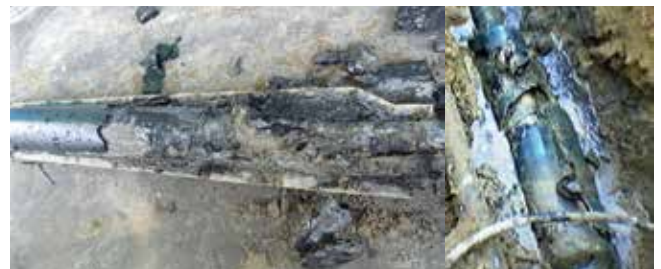
➤ vaporized core after cable fault, 132 kV XLPE
