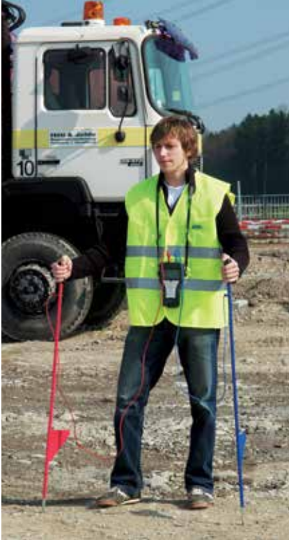
➤ step voltage method, two earth probes connected to UL30 receiver
