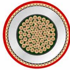
➤ Shielded concentric middle to high voltage cable, 1 conductor plus shield, faults between core and shield.
