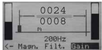
➤ UL30 display, manhole mode, display of two propagation time values used for distance calculation
