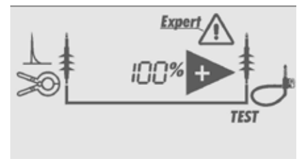
➤ KSG receiver display indicating direction, value, line conductivity
