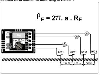
Selective measurement at high voltage pylons:
