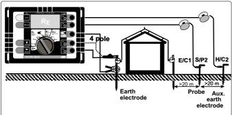
Earth resistance measurement at high voltage pylons:
