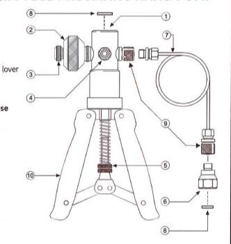
The system is a portable dual source of vacuum and pressure. Each system incorporates a vacuum / pressure selector, a volume control for fine adjustment and adjustable stroke to provide over pressure protection.
