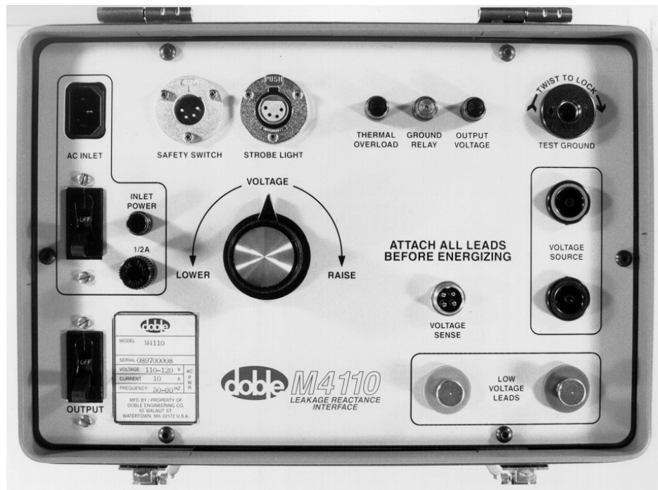
Figure 1.8 M4110 Leakage Reactance Interface
