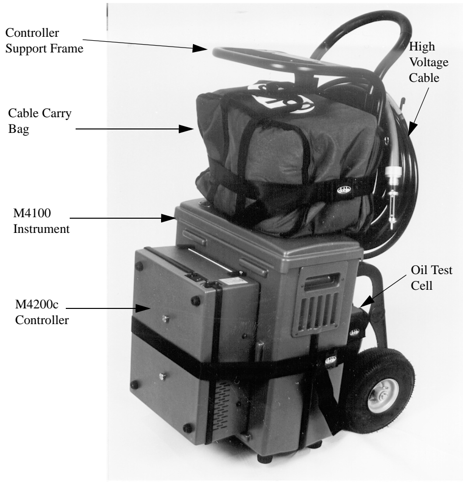
Figure 1.9 M4000 Insulation Analyzer in Storage Mode
