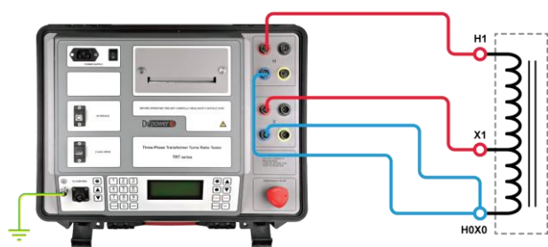
Connecting TRT to a single-phase autotransformer
