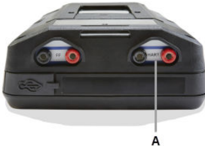
Figure 3-8: HART communication terminals on the Device Communicator communication module
