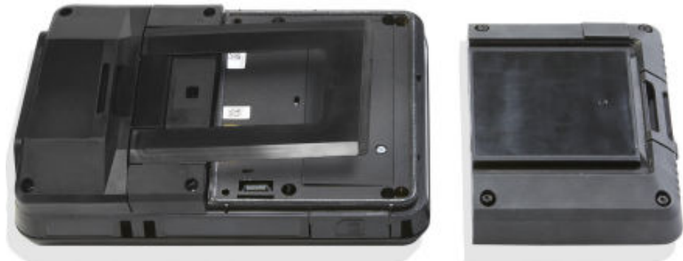
Figure 2-10: Trex unit with the power module removed
