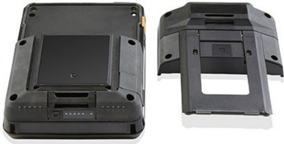
Figure 2-7: Trex unit with the communication module removed
